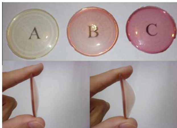
Figure 1. Photograph of the flexible bridged polysilsesquioxane plastic films undoped SSO (A) and doped SSO-P with 550 \mu L (B) and 1100 \mu L (C) of P-acid 4 \times 10^{-4} M stock solution in THF.
